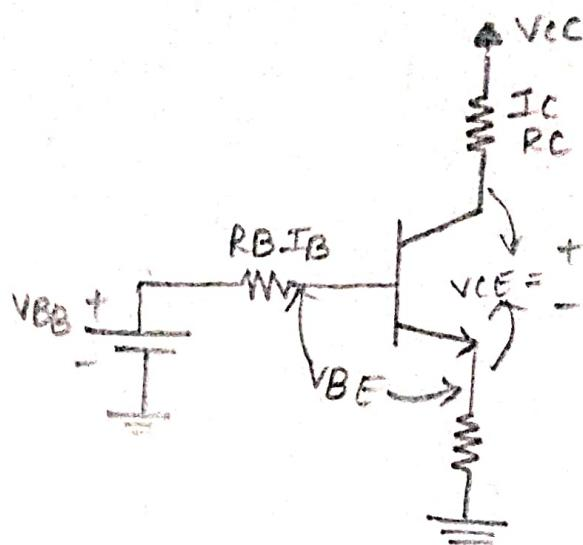
6. Determine the Quiescent values of  $i_b$  as shown in following circuit diagram assume that  $\beta = 100$  and  $V_{BE}$  is 0.7V.
