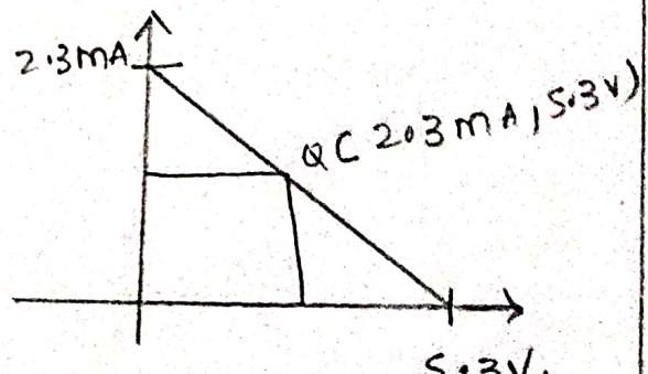
Q. Examine the operating point in a silicon transistor with a fixed bias,  $V_{CC} = 9V$ ,  $R_C = 3k\Omega$ ,  $R_B = 1M\Omega$ ,  $\beta = 200$ ,  $V_{BE} = 0.7V$
